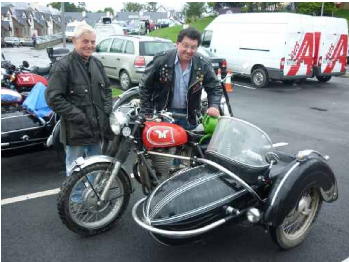
Two happy faces as Justin is at work with the water can again & Brian keeps his hands warm. Due to the oil leak out of the magneto drive cover, nearly two watering cans of oil were needed.
